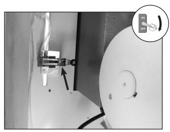
Figure 49. Blade release switch.
